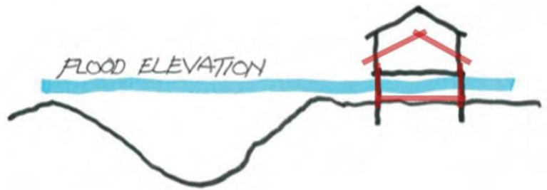
Figure 13: Graphic illustration elevation of structure
