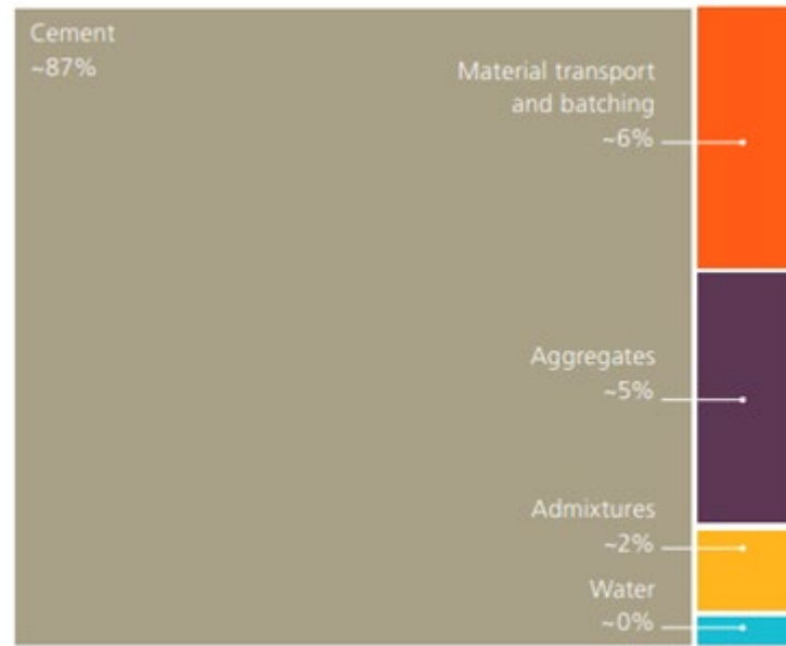
Fig 1.1: Distribution of embodied carbon in a typical structural concrete (RC25/30), LCA stages A1 to A3
